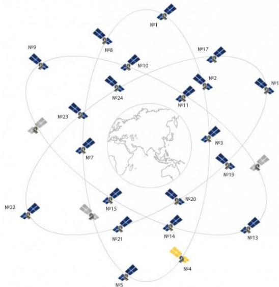
Figure 3.19: This figure shows the GLONASS Orbital Planes. These are meticulously assigned to assure that receivers in all areas of the world can track their positions. The orbit of GLONASS different than that of GPS.
